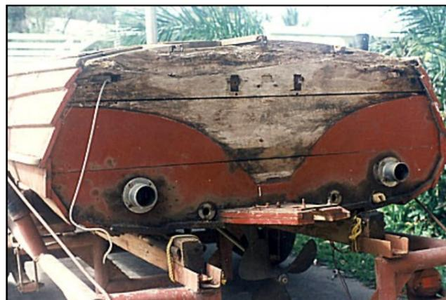
Glenn has been busy since July. The hull has been stripped down and the paint removed. Two lower planks have been repaired and two lengths of planking on the sides were replaced because of some
