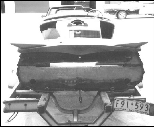
The day the boats was picked up - cav plate torn off and holes in the transom
