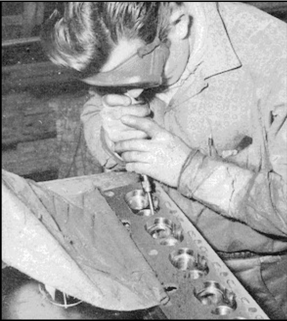
Porting and polishing is a highly skilled art. Here a competent mechanic uses a high speed drill to polish valve seats. The piece of cloth fixed to the left has two purposes, to stop the glare of light from the bulb lighting the work area shining into the operator's eyes, and to keep dust and grindings down.
